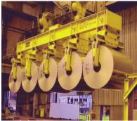
5 Coil Lifters-1 Spreader Beam
