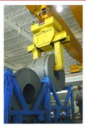
Coil grab features include motorized or manual adjustment, low headroom designs, replaceable wear bars for high duty cycle operation, optical sensors, full length coil sensing flapper assemblies on drop legs, protective padding and rollers, special bail configurations, motorized rotation and built-in weigh scales.
