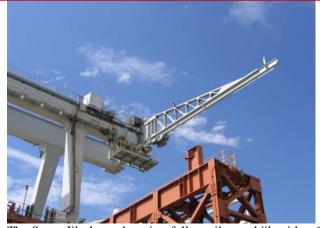
The Super Jib shown here is a full cantilevered jib with a 60-foot span and a capacity of 7 ½ tons. It is mounted onto a large gantry crane at a nuclear power plant in California.
