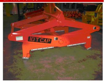
Avon Engineering designs and manufactures a complete line of tongs for lifting and moving industrial loads with capacities from 50 pounds to 100 tons. Tongs are custom designed to suit your applications including work rolls, billets, slabs, pipes, bar stock, concrete, etc. at high or low temperatures.
