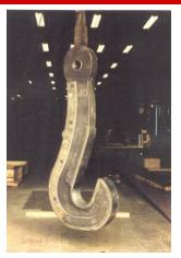
Ladle beams with ladle hooks or J-hooks are used to transport a ladle and allow the ladle to be rotated. Features include:
