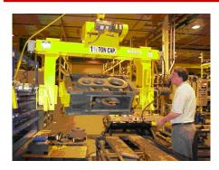
Rotating axis grabs grip the outside of a load and rotate it to the proper position. They are ideal for applications involving loads that are packaged or banded. They can be operated manually or powered by an electric or air motor.
