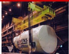
This 230-ton capacity beam lifts a \$21 million dollar turbine. The beam is custom designed to pick up engines with various configurations.
