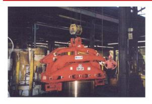
Vertical rim coil lifters lift coils in the eye-vertical position to permit stacking for heat treating processes. Vertical rim coil grabs are available for single rim and double rim applications.
