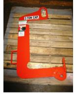
The C-hook above was engineered to move small palletized slit coils (mults) from eyehorizontal to eye-vertical position. It is made of high strength steel with inside corners polished and NDT inspected and is available in capacities from 500 to 10,000 pounds.
