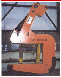
Spring balanced C-hooks are particularly useful for handling large coils. By eliminating the need for a counter weight, they minimize the weight of the hook. Coil edge protection is available.
