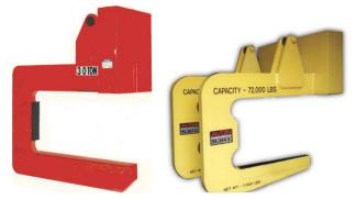
These C-hooks are designed for close stacking. The distance from pick-up point (center of gravity) to the end of the hook is shortened. The shorter lifting arm permits handling all coil widths within operating range (widest to narrowest) without the lifting arm extending beyond the outer edge of the coil.
