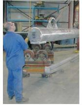
This C-hook was designed for submerging wire or rod coils in an acid pickling line. It is clad in 100% nickel to protect the steel used in the fabrication of the units.
