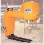
This combination C-hook and pallet lifter is a versatile unit that can handle both coils and palletized materials. It can be designed with either motorized or manual fork adjustment.
