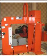
Since C-hooks are large and heavy, they can cause personal injury or property damage if they fall over. Each C-hook should be stored in an upright position on a stand specifically designed for its size, shape and weight.
