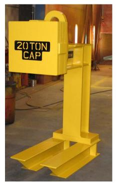
The Model 900 fixed fork pallet lifter utilizes stationary forks to handle palletized loads of various configurations.
