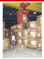
Avon Engineering builds higher capacity pallet lifters with a double vertical member.
