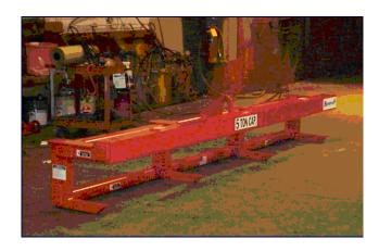
Pallet lifter modified to lift billets
