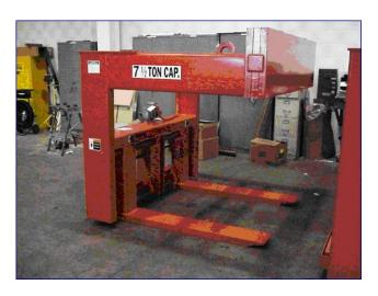
An electric motor adjusts the forks on this lifter
