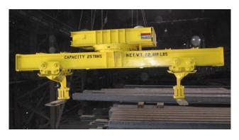
25-ton capacity spreader beam with powered rotation and lifting forks with adjustable spacing for handling hot beam
