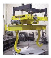
This rotating beam has adjustable J-hooks and an integral weigh scale system.
