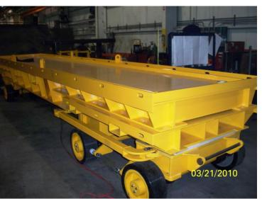
60,000 pound capacity towable tube bundle cart. The cart has a hydraulic braking system.
