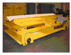
This 50-metric ton capacity coil transfer car can transport two 25-metric ton coils. Replaceable wear pads protect the coil surface. The operator walks along with car, operating it from a hand-held pendant.
