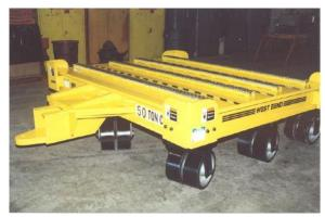
Fabricated of heavy-duty welded steel, this non-powered, towable die cart is a durable and inexpensive addition to your die-transport operation. The top platform is fitted with super-rail low friction roller sections for easy die transfer. It features a fabricated steel hitch pin so that a forklift can move it easily around the plant.
