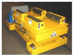
This Avon Engineering scissors lift coil transfer car has power rotation. It is rated for 15,000-pound capacity and is designed to handle aluminum coils, 62" by 56" wide. The coil is supported by gravity type rollers to permit proper coil tail orientation.
