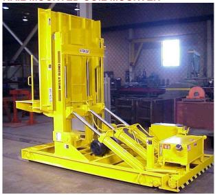
Rail mounted coil cars can handle a full range of coil sizes and weights. This multi-function machine will:
