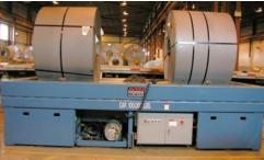
Propane powered transfer cars are used for handling coils, dies and molds.
