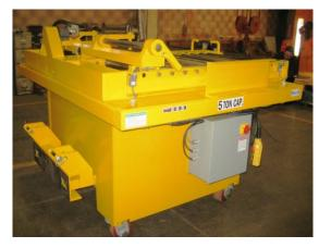
This five-ton capacity, towable mold cart has a hydraulically powered mold transfer deck.
