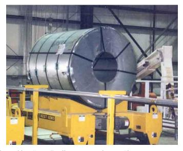
These fully automated coil transfer cars are track mounted and located in a "green" coil storage warehouse. They were designed to move steel coils weighing 42 tons, up to a maximum diameter of 80 inches and a maximum width of 72 inches. There are five cars in this facility.
