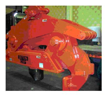
The Model 6100 Single Rim Vertical Coil Tong handles coils by gripping the ID and OD on one side of the coil. Gripping force is more than three times the coil weight.
