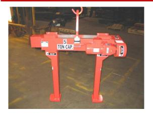
This is a motorized version of the Model 2020. It can be used in high volume operations where stacking heights can be high.
