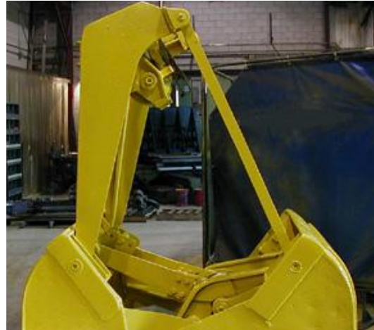
One cubic yard, single line clamshell bucket
