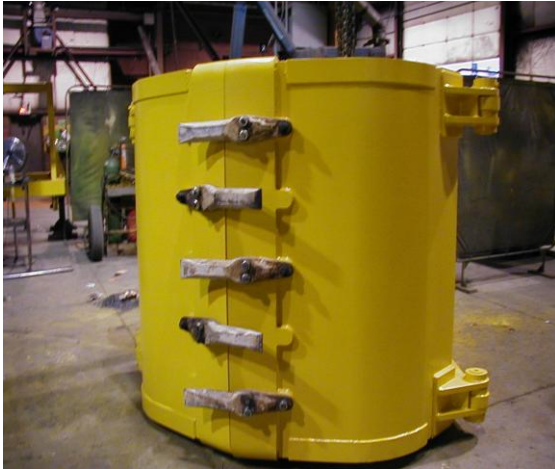
Clamshell bucket with replaceable digging teeth
