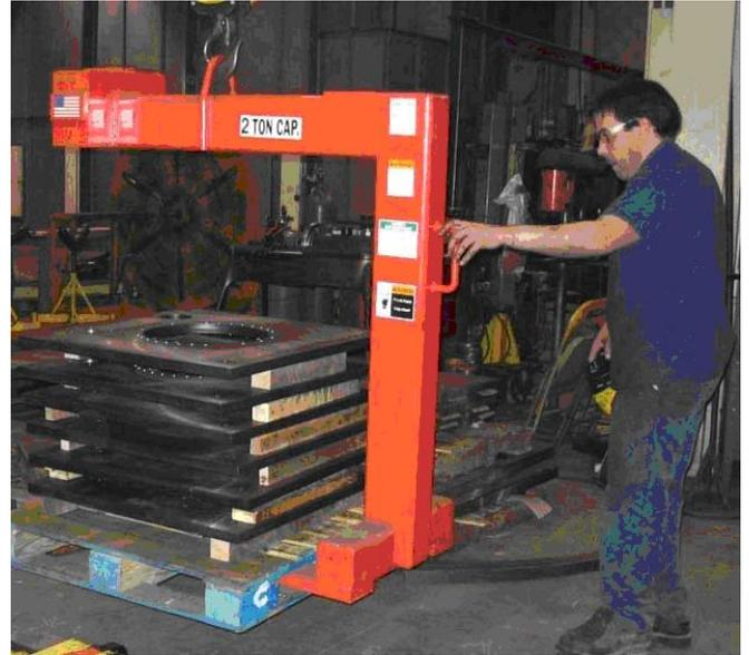
Avon Engineering pallet lifters are available in capacities from 500 pounds to 20 tons. Pallet lifter features include:
