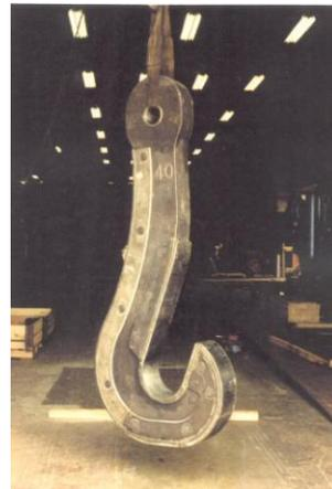
Ladle beams with ladle hooks or J-hooks are used to transport a ladle and allow the ladle to be rotated. Features include:
