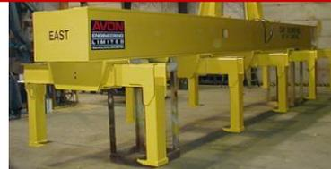
Sheet lifters feature hand wheels, chain wheels and motorized leg travel. They can be equipped with low profile designs; end hooks; load weighing systems; and self-locking leg designs that prevent opening under load.
