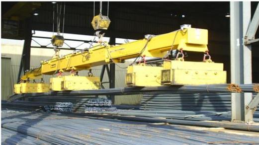
Magnet beams feature twin bail pick-up, fixed length or motorized telescopic Tri-Beam, and hardened steel bushings at magnet attachment points. Beams are available with built-in storage stands.
