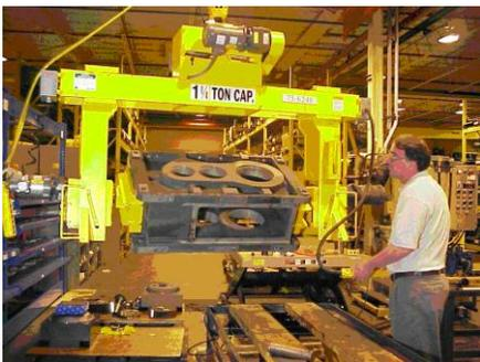
Rotating axis grabs grip the outside of a load and rotate it to the proper position. They are ideal for applications involving loads that are packaged or banded. They can be operated manually or powered by an electric or air motor.
