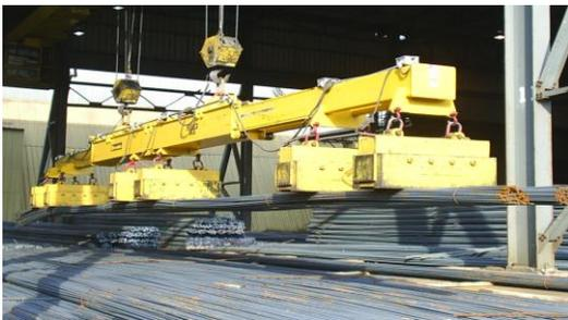
Magnet beams feature twin bail pick-up, fixed length or motorized telescopic Tri-Beam, and hardened steel bushings at magnet attachment points. Beams are available with built-in storage stands.
