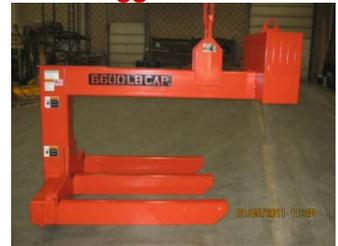
Designed for lifting three hot forgings at once
