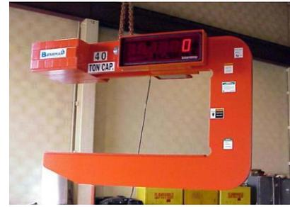
Avon Engineering C-hooks can also be equipped with integral load weighing systems. The accuracy of the load cells is from plus or minus 0.2% to 0.5% of full load. The calibration settings are saved in memory even during loss of power. All Avon Engineering C-hooks are designed and manufactured in accordance with ASME Spec. B30.20 and BTH-1: Design of Below-the-Hook Lifting Devices.
