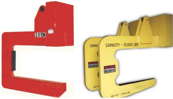
These C-hooks are designed for close stacking. The distance from pick-up point (center of gravity) to the end of the hook is shortened. The shorter lifting arm permits handling all coil widths within operating range (widest to narrowest) without the lifting arm extending beyond the outer edge of the coil.
