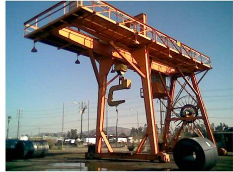
Mill duty C-hooks are built with larger sections and corner radii to keep stresses to a minimum, thereby providing maximum service life.
