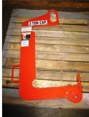
The C-hook above was engineered to move small palletized slit coils (mults) from eye-horizontal to eye-vertical position. It is made of high strength steel with inside corners polished and NDT inspected and is available in capacities from 500 to 10,000 pounds.
