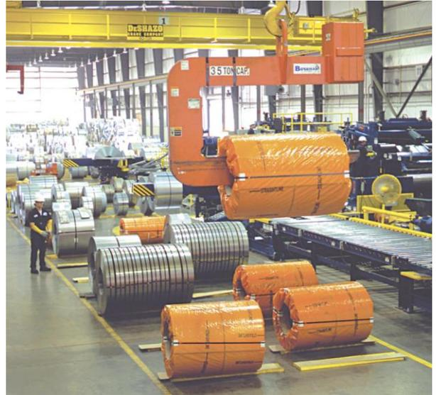
All Avon Engineering C-hooks are designed and manufactured in accordance with the latest revisions of ASME Specifications B30.20 and BTH-1, Design of Below-the-Hook Lifting Devices.
