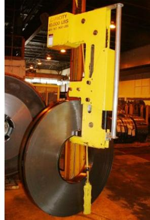
Faster and safer than a conventional C-hook, this specially designed lifter facilitates fast and safe placement of a slit coil onto an un-coiler mandrel. It adjusts automatically to varying coil diameters. The full length handle makes it easier to maneuver the lifter.
