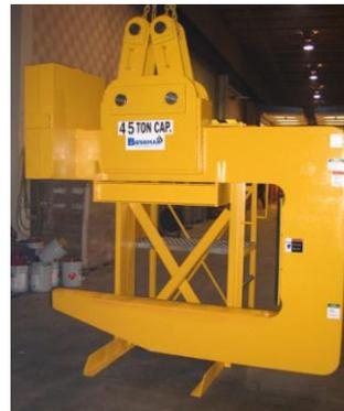
Since C-hooks are large and heavy, they can cause personal injury or property damage if they fall over. Each C-hook should be stored in an upright position on a stand specifically designed for its size, shape and weight.
