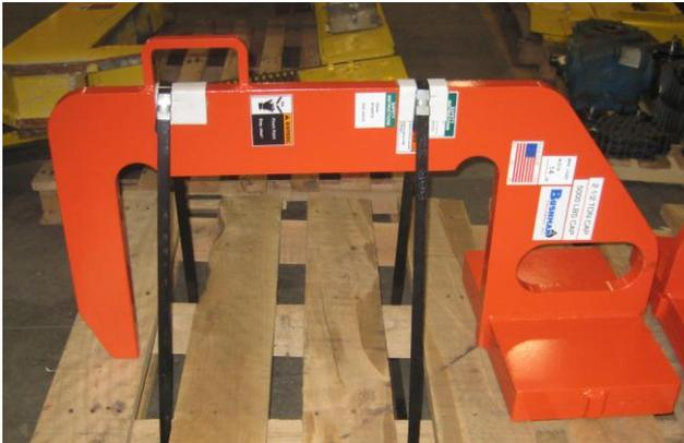
The Model 610 C-hook is similar in construction to the Model 624. The lifting bail is burned from the same piece of plate as the hook, making it an integral part of the C-hook.
