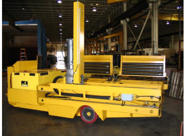
This battery powered free ranging mold cart has two 24,000 pound mold decks. The decks are raised and lowered by a scissors lift.
