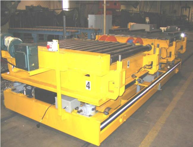
This two-station, 20,000 pound capacity, fully automated mold cart serves a line of molding machines.
