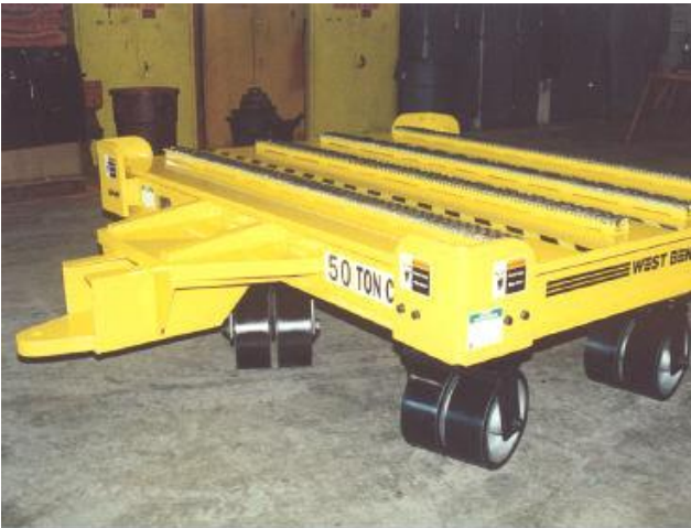
This towable die cart can handle 100,000 pound dies
