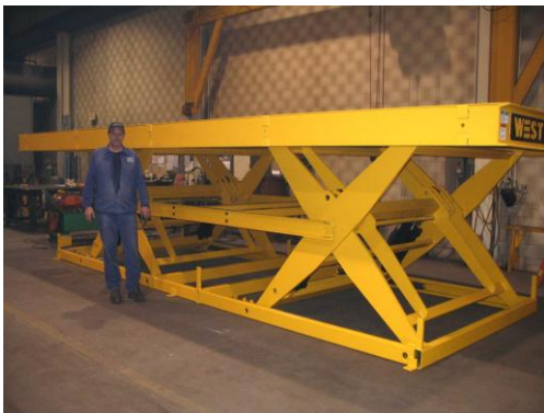
This custom double long scissors lift is used by a major flooring manufacturer to index sheets of linoleum flooring.
