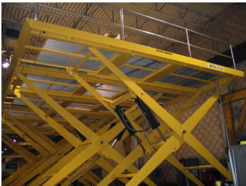
This 12,000-pound capacity scissor lift table platform is 23' x 44' and is used in a commercial jet engine test cell.
