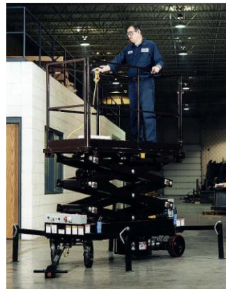
These 1,000 pound, hydraulically operated aerial maintenance lifts are dependable, affordable and generally maintenance free. They can pass through 36-inch doorways and fit into standard elevators for use in multi-story buildings. In spite of their high capacity, they are light weight and easy to transport between work sites.
