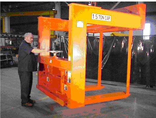
The model H-901, an adjustable fork pallet lifter, permits the operator to move the forks with a hand wheel or hand crank. This ergonomic feature improves operator efficiency and safety. This option is highly recommended for pallet lifters with capacities over 6,000 pounds and is standard on all models over 10 tons. The fork adjustment mechanism can also be motorized. For information about special options and sizes, please call the factory or your local sales representative.
