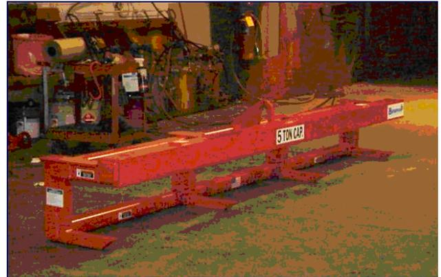
Pallet lifter modified to lift billets
