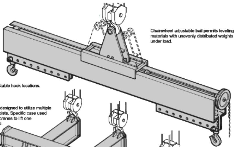
Chainwheel adjustable bail permits leveling materials with unevenly distributed weights under load.
