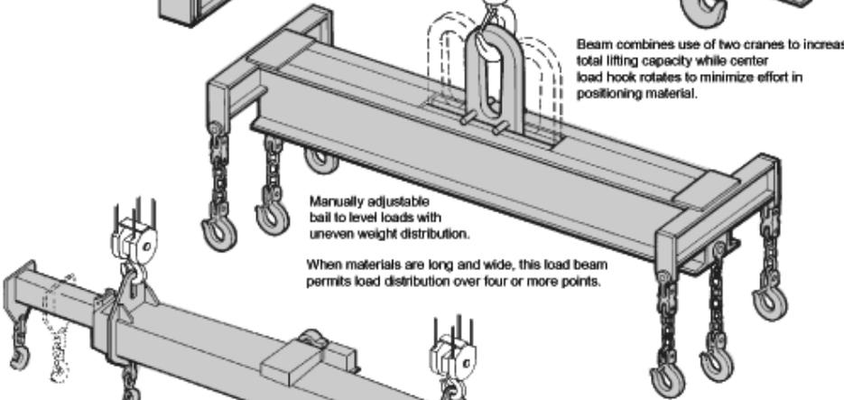
Beam combines use of two cranes to increase total lifting capacity while center load hook rotates to minimize effort in positioning material.
