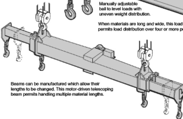
Beams can be manufactured which allow their lengths to be changed. This motor-driven telescoping beam permits handling multiple material lengths.
