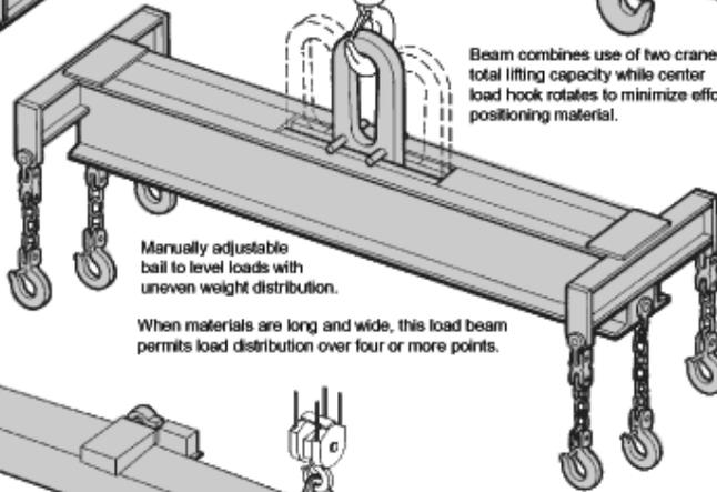
Manually adjustable bail to level loads with uneven weight distribution.
