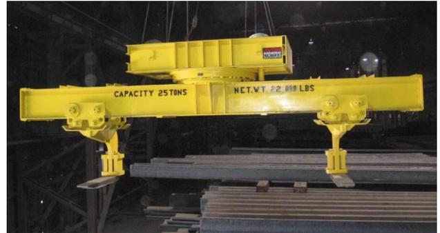
25-ton capacity spreader beam with powered rotation and lifting forks with adjustable spacing for handling hot beam
