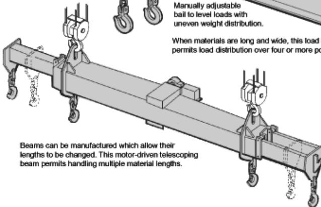
Beams can be manufactured which allow their lengths to be changed. This motor-driven telescoping beam permits handling multiple material lengths.
