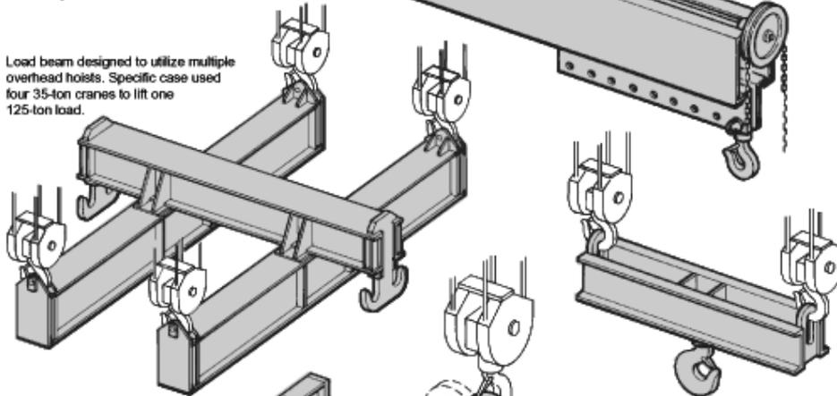
Load beam designed to utilize multiple overhead hoists. Specific case used four 35-ton cranes to lift one 125-ton load.
