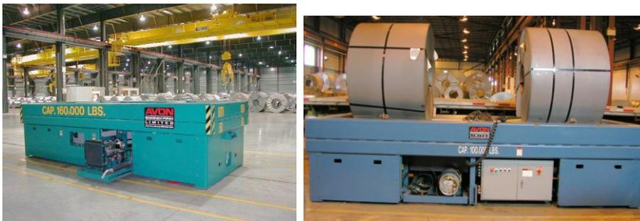
Propane powered transfer cars are used for handling coils, dies and molds.
