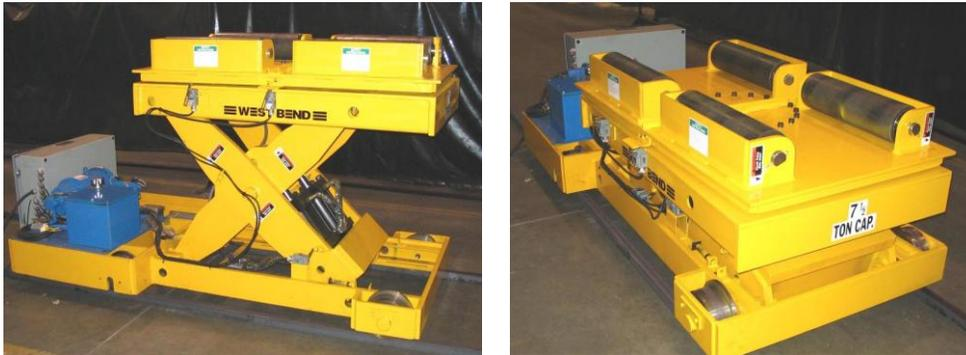
This Avon Engineering scissors lift coil transfer car has power rotation. It is rated for 15,000-pound capacity and is designed to handle aluminum coils, 62" by 56" wide. The coil is supported by gravity type rollers to permit proper coil tail orientation.
