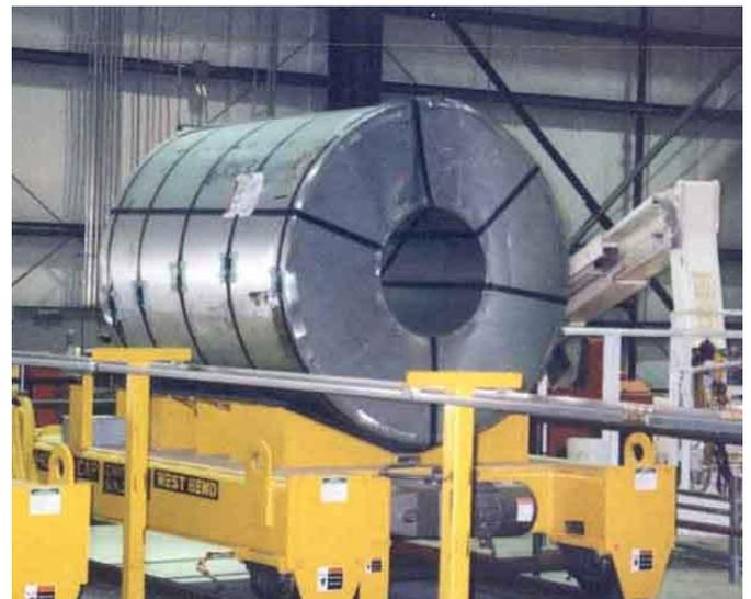
These fully automated coil transfer cars are track mounted and located in a “green” coil storage warehouse. They were designed to move steel coils weighing 42 tons, up to a maximum diameter of 80 inches and a maximum width of 72 inches. There are five cars in this facility.
