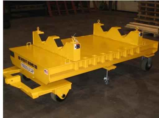
This 10,000 pound capacity cart is towable and has V-blocks that can be adjusted to the desired load length.
