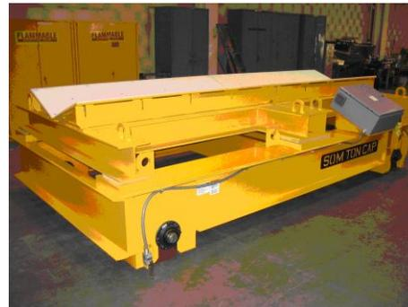
This 50-metric ton capacity coil transfer car can transport two 25-metric ton coils. Replaceable wear pads protect the coil surface. The operator walks along with car, operating it from a hand-held pendant.
