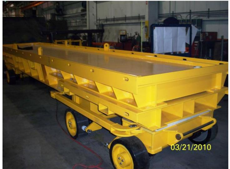
60,000 pound capacity towable tube bundle cart. The cart has a hydraulic braking system.
