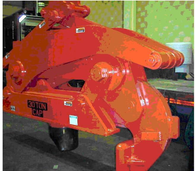
The Model 6100 Single Rim Vertical Coil Tong handles coils by gripping the ID and OD on one side of the coil. Gripping force is more than three times the coil weight.
