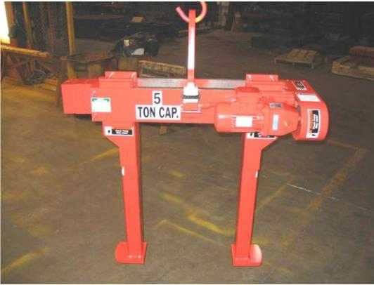
This is a motorized version of the Model 2020. It can be used in high volume operations where stacking heights can be high.
